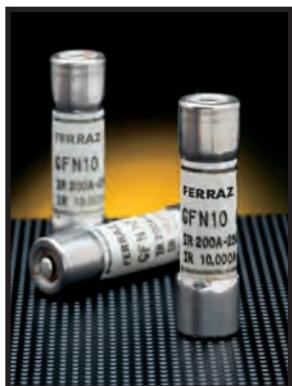
GFN midget indicating fuses are available in ratings from 1/10A through 30A. These time-delay fuses have built-in blown fuse indicators which pop out at the end of the fuse to visually indicate when the fuse has operated to open the circuit. Indicators may be used to trip a switch for remote as well as visual annunciation. (Not for Branch Circuit Protection).
