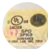
The picture to the left is of a holographic label from a UL 1449 3<sup>rd</sup> edition device. Please note the SPD wording, which is accepted in today's industry.
